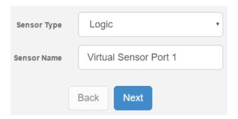
The logic is a new virtual sensor type on SP2+ which uses FlipFlop logic. You can monitor physical sensor statuses with it, and change the virtual sensor's state with the pre-set values for the status of a physical sensor (SET Source Sensor).
