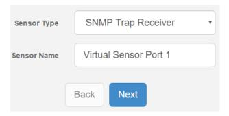
The SNMP Trap Receiver type will check 3 parameters before setting a value for the virtual sensor. These three parameters are the IP Address, the sensor's OID and the Trap sub-type.
