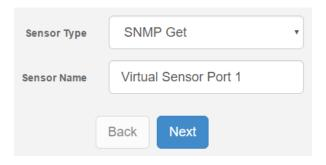
With SNMP Get sensor, you can get a value from any SNMP device. Note that a custom string return value is not supported.
