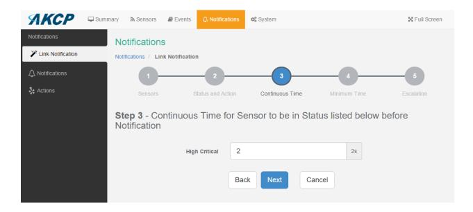
We set the continuous time as 2 seconds - this means the sensor's state has to remain at least 2 seconds in the chosen state before the notification runs.
